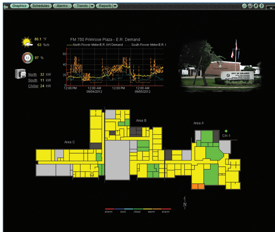
Figure 1: BAS summary graphic of Primrose Plaza, one of the larger buildings in this project. The gray areas indicate unoccupied rooms where sensors have turned off the HVAC to save energy.
