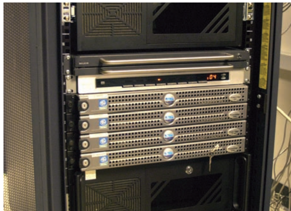
Photo 2: BACnet Web ports use the BAS software to display equipment and real-time data via a Web browser.
