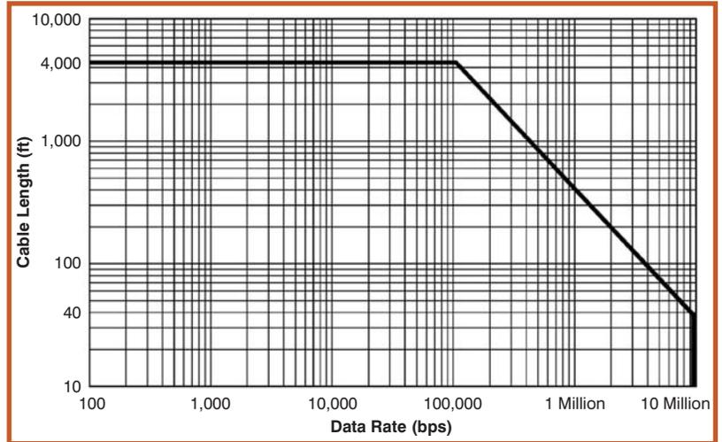
**Figure 2:** A graph depicting cable length and data rate of RS-485. Source: National Instruments Application Note 1057 “Ten Ways to Bulletproof RS-485 Interfaces.”
