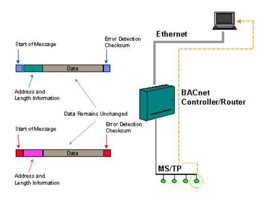
Figure 1: A BACnet router connecting an Ethernet LAN to an MS/TP LAN. The content of the message does not change even though the addressing, signaling, and framing change. In a gateway the data must also be translated.
