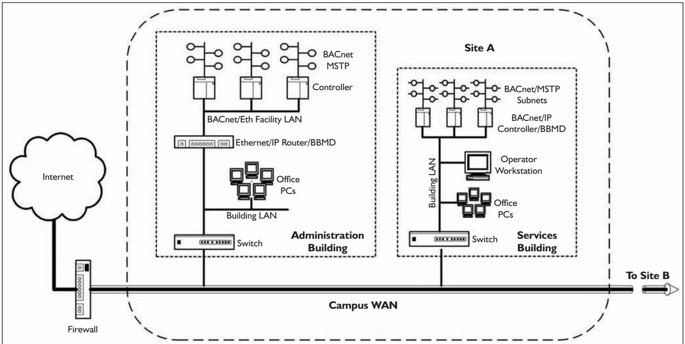
Figure 2: Campus network with facility networks using campus WAN for high-level BACnet communications.
