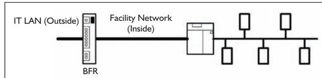
*Figure 1: BFR as firewall between IT LAN and BACnet network.*
